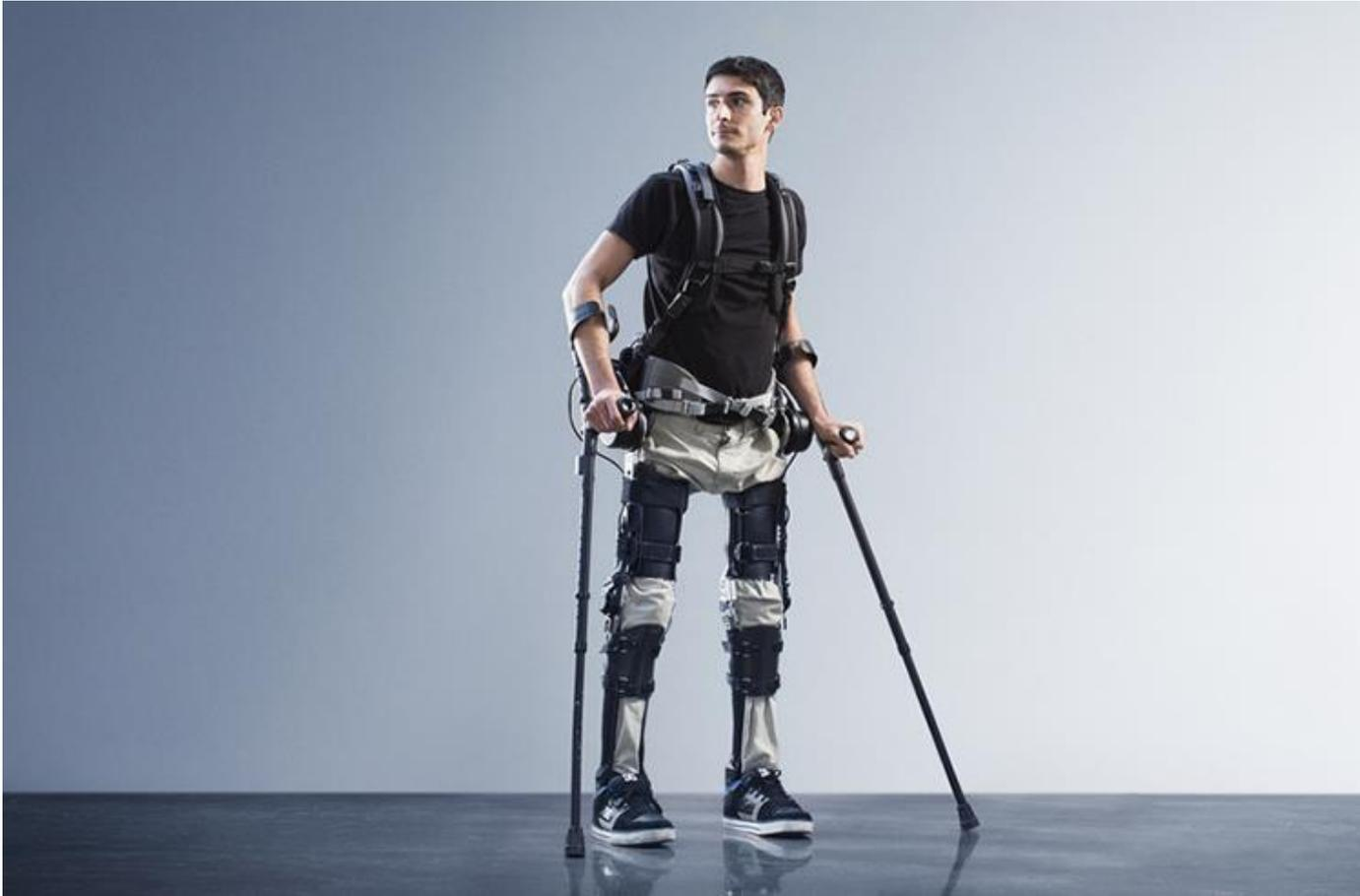
Developed from the Berkeley Lower Extremity Exoskeleton (BLEEX), the Phoenix is one of the lightest and most accessible exoskeletons available. 13
